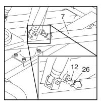
Switch and the Magnet should be about 1/8". Make sure that the Magnet will not hit the Reed Switch when the Right Pedal Leg is moved. Repeat until the console displays correct feedback.
